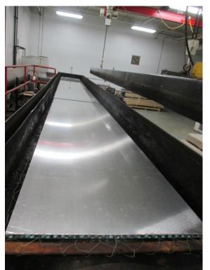
Photo No. 2 Specimen Mounted in Tunnel Unexposed Surface (Pre-Test)
