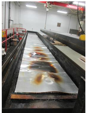
Photo No. 3 Specimen Mounted in Tunnel Unexposed Surface (Post Test)
