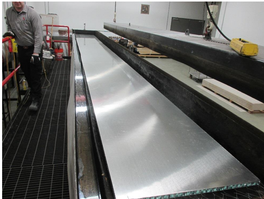
Photo No. 2 Specimen Mounted in Tunnel Unexposed Surface (Pre-Test)
