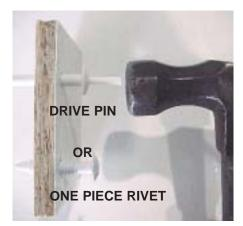
NOTE: For FRP liner panel installation, pre-drill hole 1/8" (.125") larger than the diameter of the rivet to allow for expansion.
